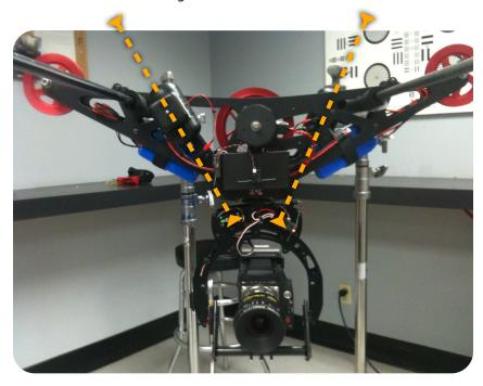
We recommend using a separate battery to spool up the gyros to proper operational speed then install the batteries you will use to run the trolley. The spool up period takes about 10 minutes. The reason to use a separate battery is because the gyros will consume more power during spooling up than at normal operation and using a separate battery other than the main trolley batteries will extend the running time of the trolley.
