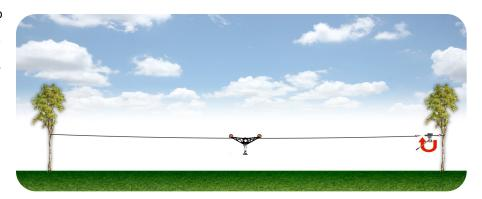
Another method is to use one fixed anchor and one movable anchor. The movable anchor is usually a heavy duty scissor lift, forklift, crane, etc. In this manner you attach the cable to the fixed anchor and the movable anchor and 'drive' the movable anchor backwards to apply proper tension on the cable.
