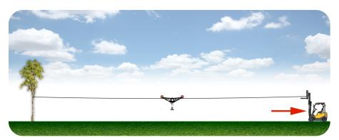
Dyneema/AMSteel rope will usually require re-tensioning once or twice after initial tensioning. This is normal and is due to it stretching slightly. Keep watch of the sag and as it increases re-tension the cable accordingly.
